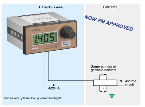
**The BA405C** is an intrinsically safe panel mounting manual set point station that enables the current flowing in a 4/20mA loop to be manually adjusted from within a hazardous area. The instrument is loop powered and contains a  $3\frac{1}{2}$  digit display which may be calibrated to show the 4/20mA current in engineering units.
